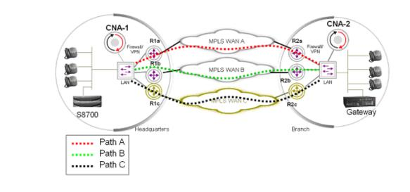
Figure 93: Enterprise example: headquarters and branch connected using 3 diverse paths
